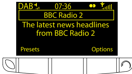
The context-sensitive buttons, with two on-screen choices, Presets and Options
